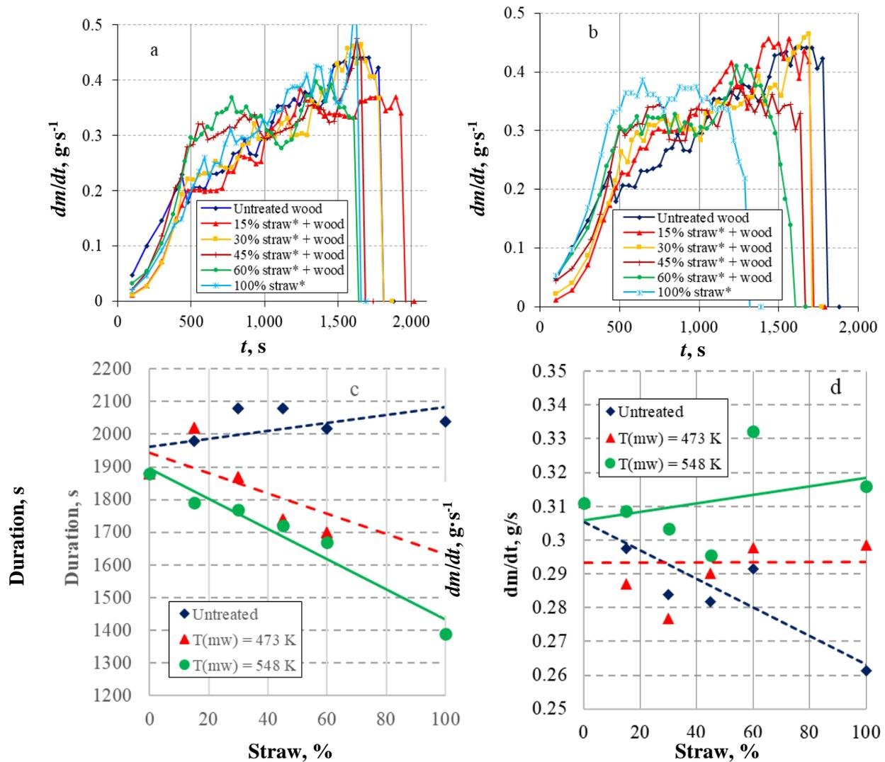
Fig. 2. Effect of variations MW pre-treatment temperature and mass fraction of pre-treated wheat straw pellets in blends with raw wood pellets on: a – weight loss kinetics ( $T = 473$  K); b – weight loss kinetics ( $T = 548$  K); c – duration of the thermal decomposition; d – average values of the weight loss rate
